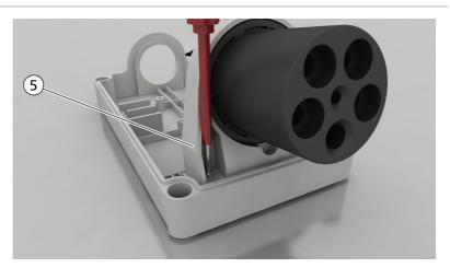
8. The terminals are open at the time of delivery. Guide the bare individual conductors into the opening and tighten the screws (6) with the minimum torque (design 63 A, contact screws M5: at least 2.0 Nm; design 125 A, contact screws M10: at least 4.0 Nm). Take care to see that only the bare individual conductor (without insulation) is clamped. Pay attention to the marking of the terminals and ensure that the assignment of the individual conductors to the terminals is correct.
